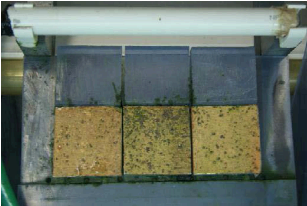
Figure 11. Test of colonization by algae on GRC samples
